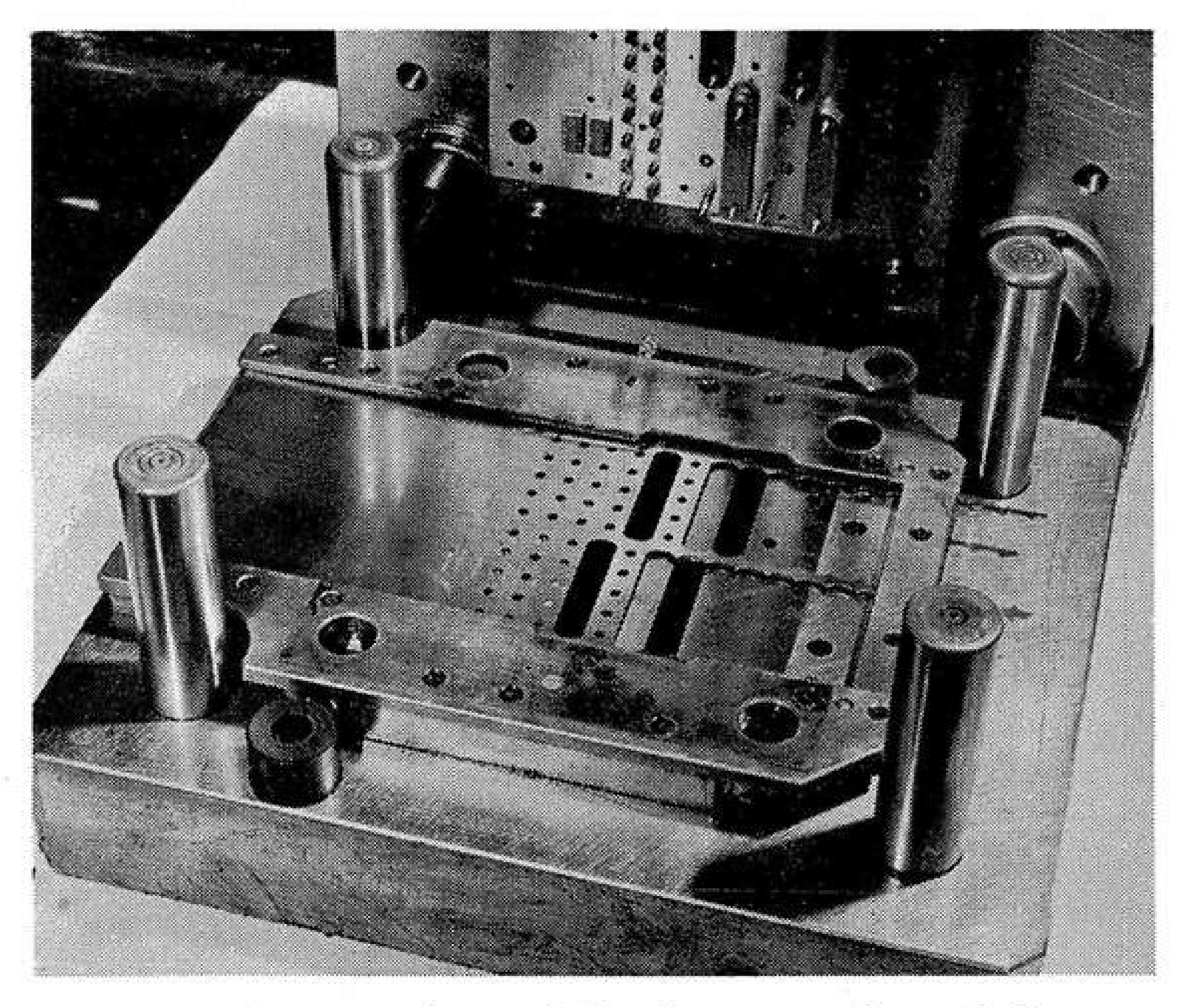
Above, a close-up view of the lower section of the new 2½" Strip press tool with a sample length of raw material in position. Note that the holes are punched before the Strips are blanked out. Below, the complete press tool. Right, a comparison between the old Strip (top) and the new.
