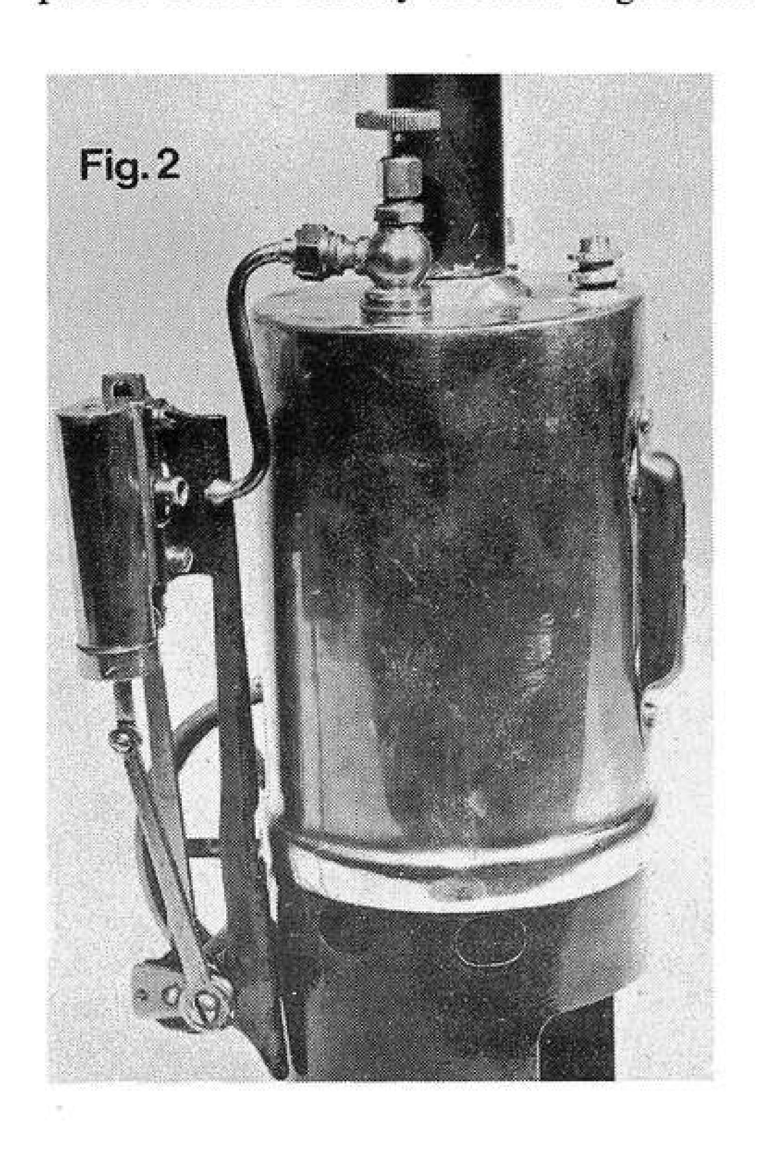
shows a general view of the firstever Meccano Steam Engine, believed to be of 1914 vintage. A very rare item, indeed, the Engine illustrated was kindly loaned to the author by Mr. Jim Gamble of Kinoulton, Notts. Fig. 2, left, shows a close-up view of the cylinder and valve gear. Note the port holes on the eccentric piston.
