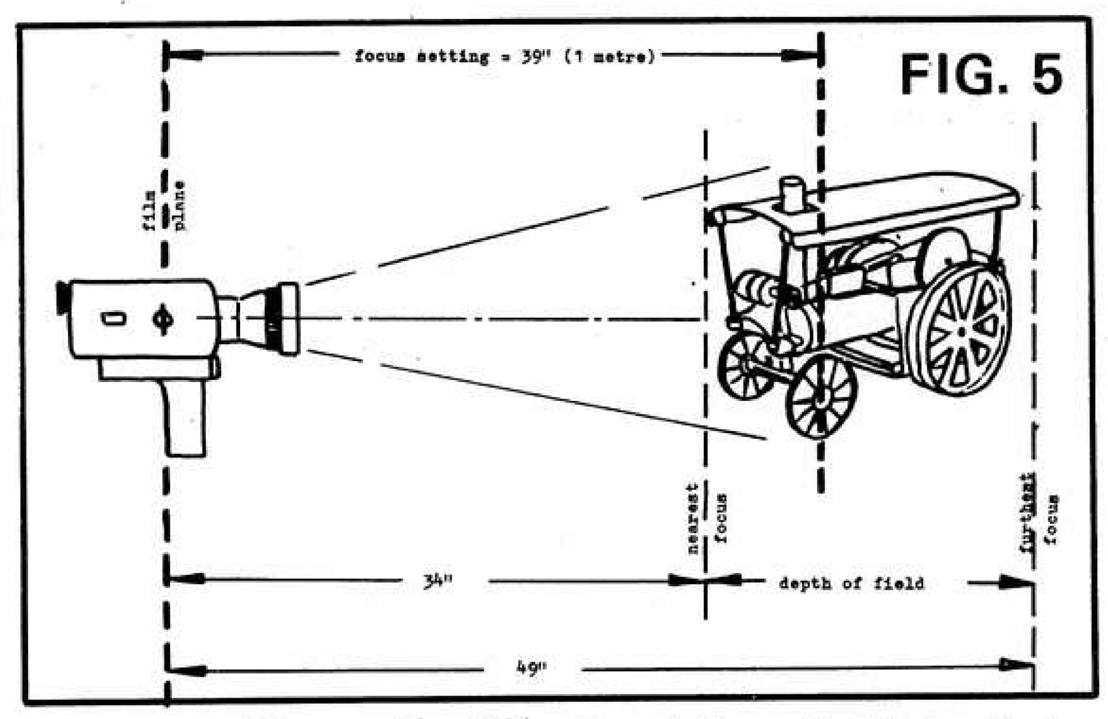
A diagram illustrating "depth of focus". Note that a greater area remains in focus behind the focussing point than in front of it.
