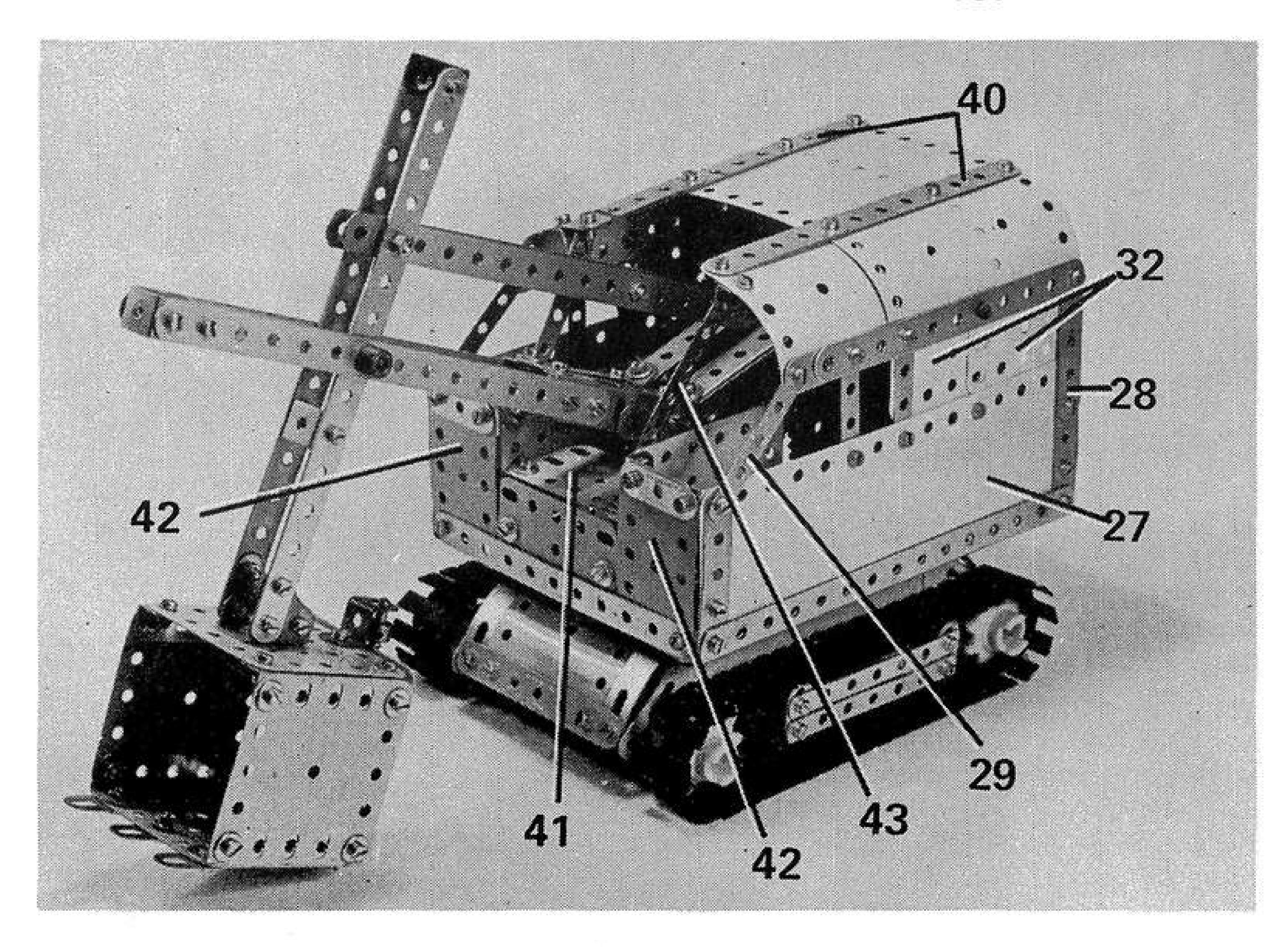
A general view of the completed Automatic Excavator described in this article. Hand-operated, it runs on crawler tracks.
