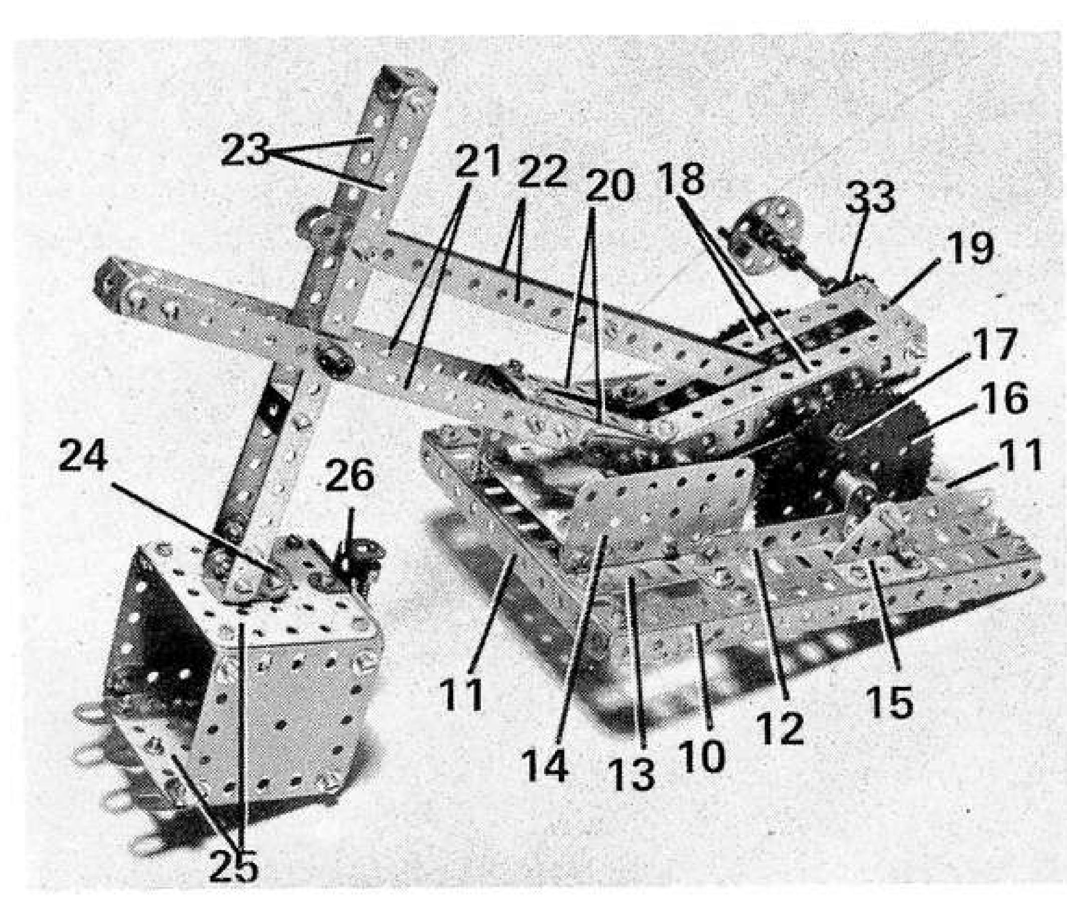
The boom and operating control mechanism removed from the Excavator. This section of the model can be assembled as a separate unit and the body then built round it. In the completed model, of course, the control wheel at the far corner of the unit would be positioned outside the body.
