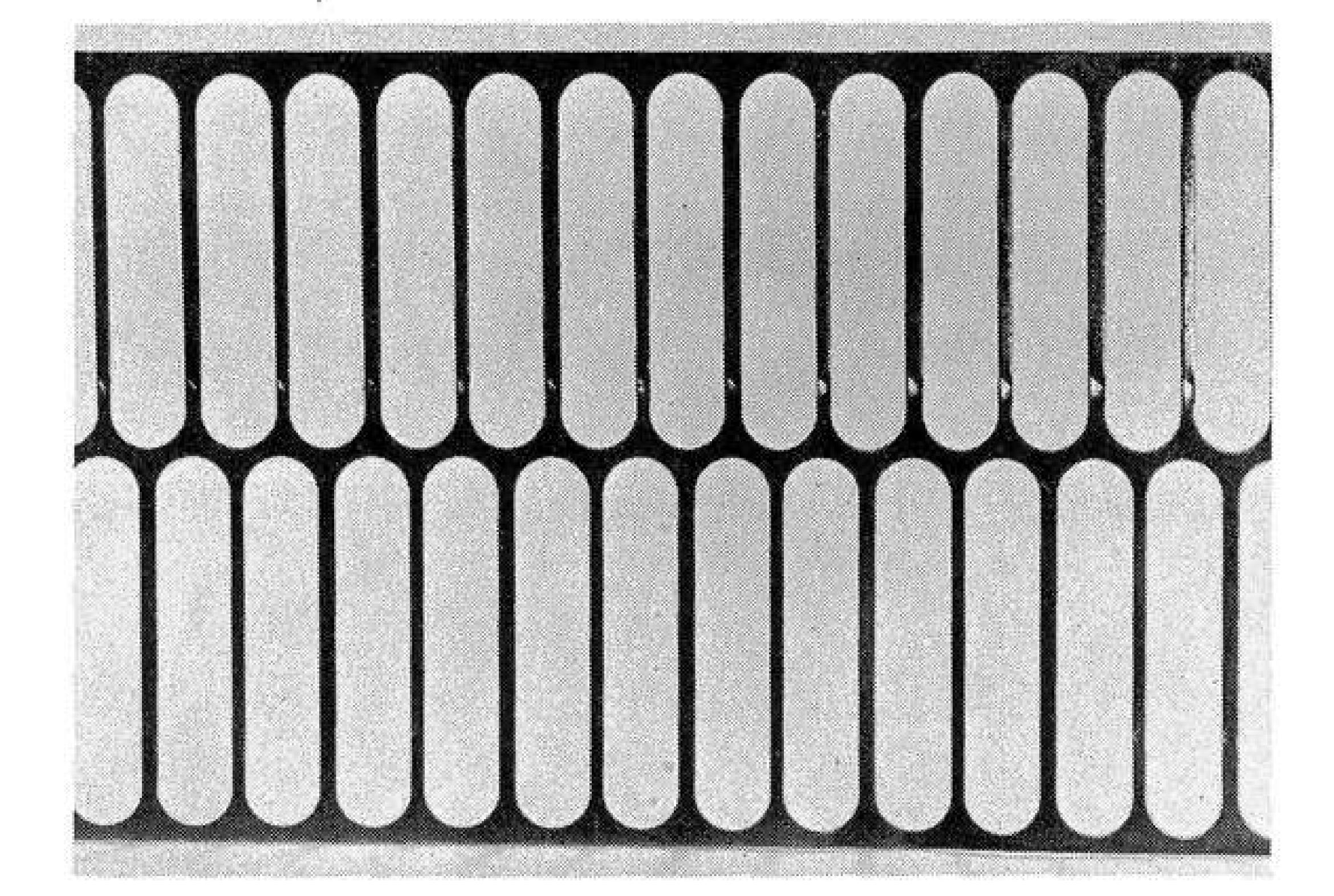
Above, a sample of raw material scrap remaining after production of the old 2½" Strip. Compare it with the tremendously-reduced scrap quantity (below) resulting from the new production method. The lower picture also illustrates that the Meccano name and the holes are punched before the Strips are finally blanked out.
