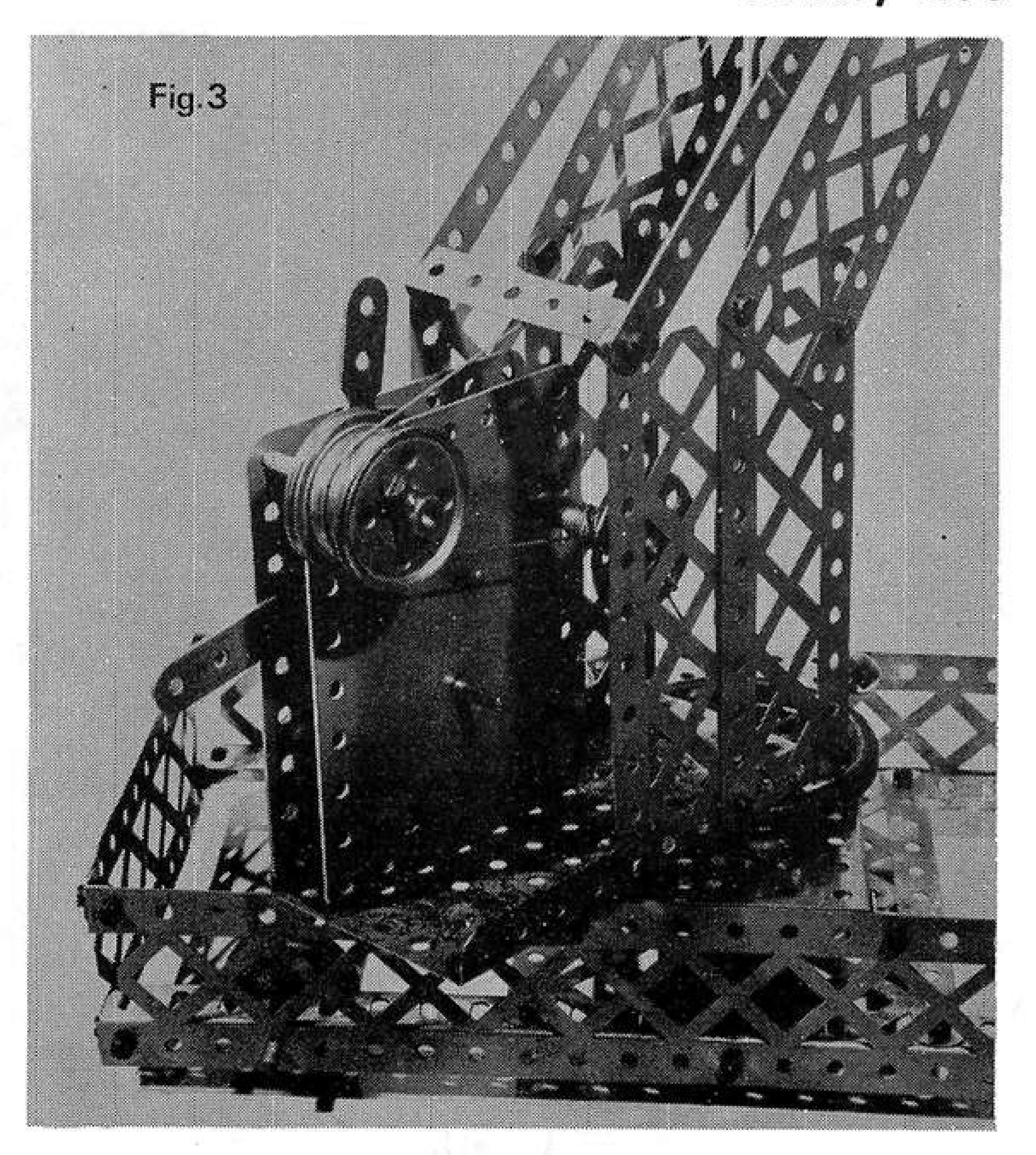
Fig. 3, a close-up view of the Crane showing the winding gear utilising the No.1 Clockwork Motor. The Author's baseplate of the period is now showing a little wear — but not bad considering the age of the part!
