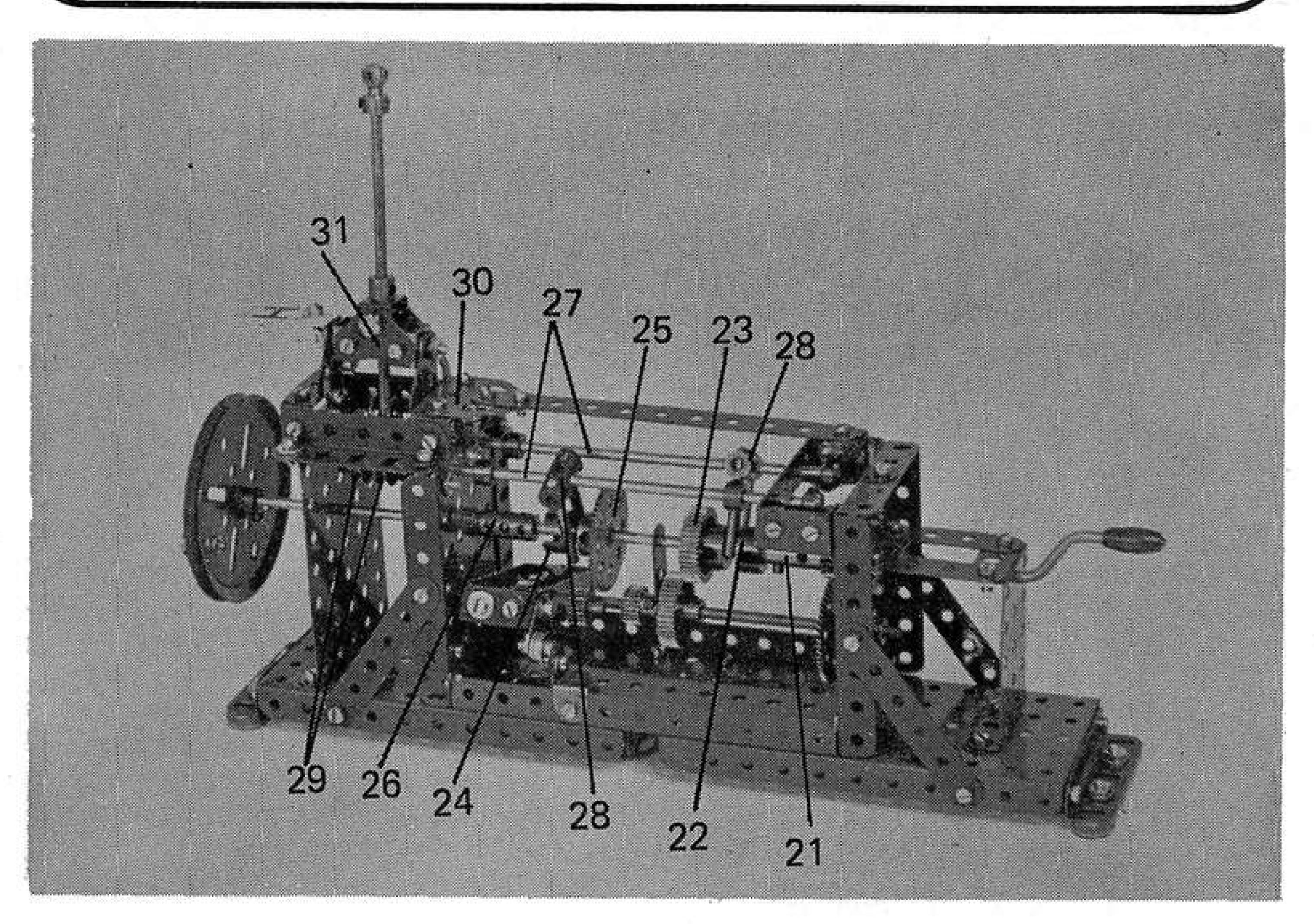
Above, a 3-speed and reverse Gearbox designed as a teaching demonstration unit by Mr Adrian Hall of Liverpool. It features an operating "H-gate" gear-change movement. Below left, a Meccano subject new to 'Spanner' is this Photographic Enlarger designed and built by Mr G. Haydn-Davies of Arnold, Notts.
