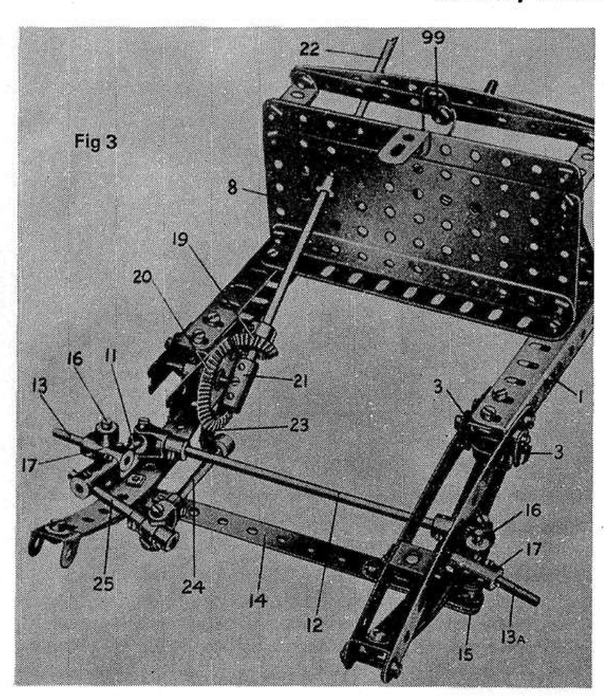
one 2½" and one 1½" Strip, placed one upon the other and slightly bent. Each end of the 5½" Strip is secured to a Double Bracket, the rear Double Bracket being bolted pivotally to Fishplates 3 and the front Double Bracket being mounted on a ¾" Bolt passed through the side frame members. Rear springs are of the cantilever type, and one of them is shown in detail in fig. 6. Each spring is built up from the same components as the front springs and is attached rigidly to the frame by Angle Brackets.
