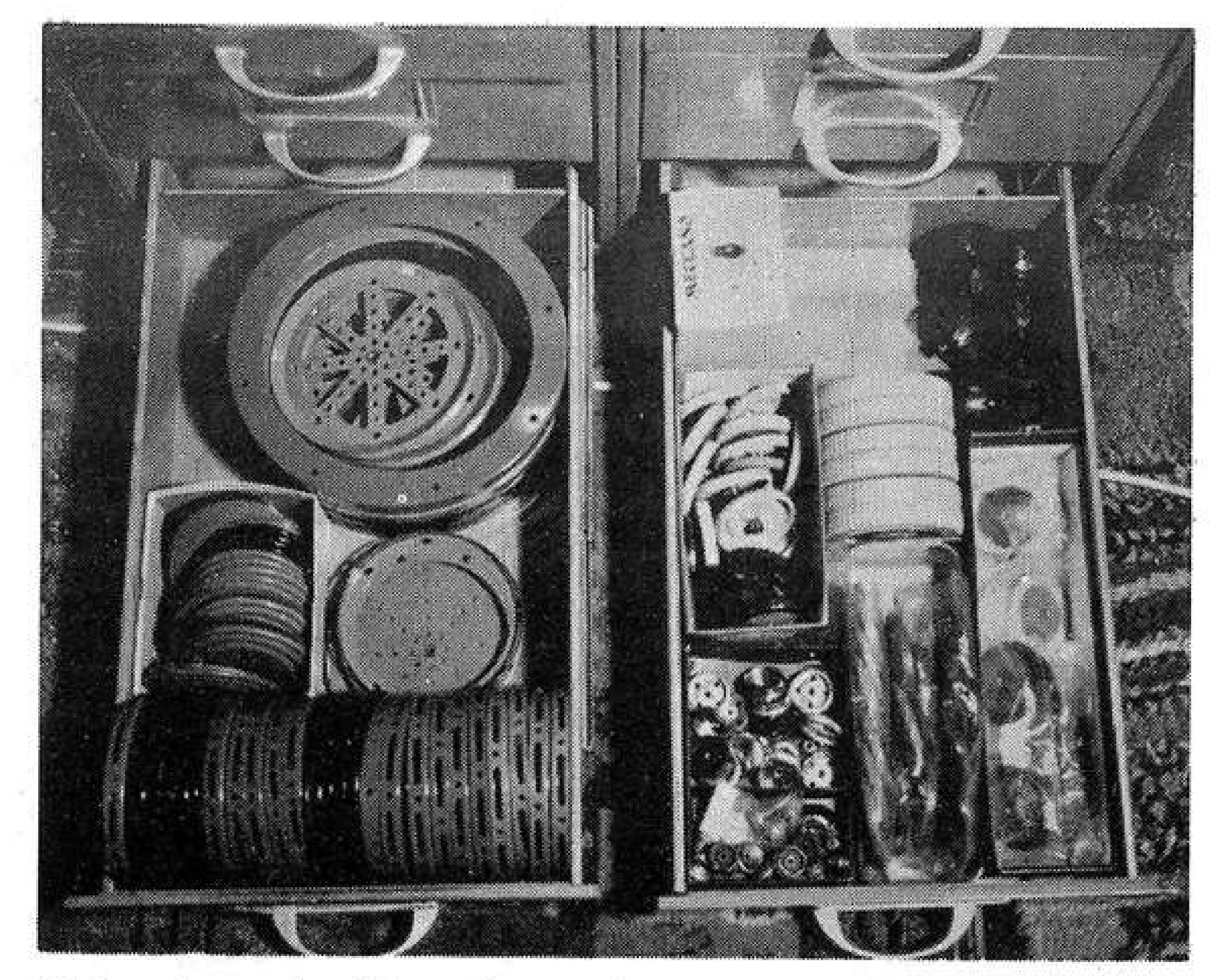
This view, looking down into two of the Author's cabinet drawers, gives a good idea of the space available by showing how easily parts such as large Flanged Rings, 6" Pulleys and Hub Discs are accommodated.
