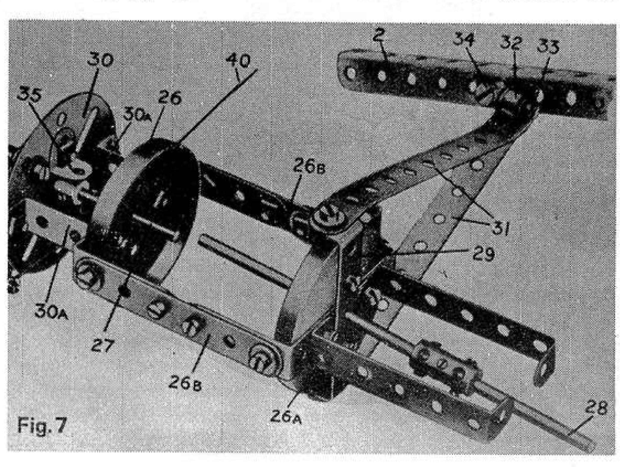
Fig. 7, a close-up view showing the back axle casing and torque rods. differential has been removed for shot. The remaining illustrations required complete the model will be included with Part 2 of the feature to be published in the next MMQ.
