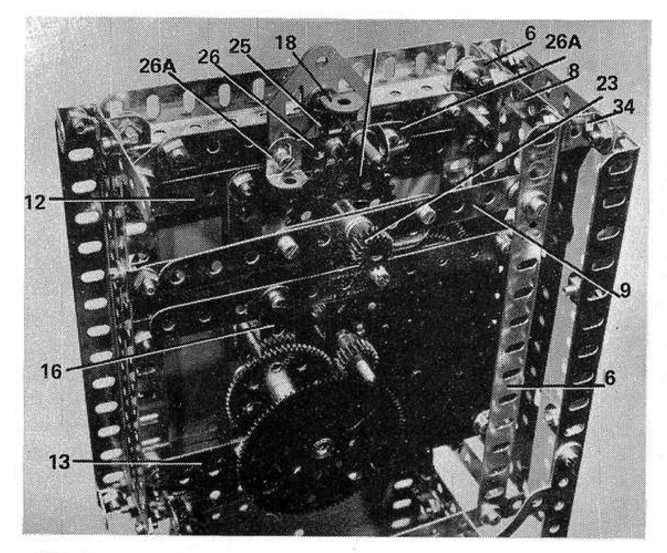
In this close-up view the Grandaughter Clock mechanism one framework Girders has been removed to allow camera to see more of the internal arrangements. The pendulum and driving 3½" Gear Wheel have also been omitted for the same reason. Construction is not as difficult as it may seem.
