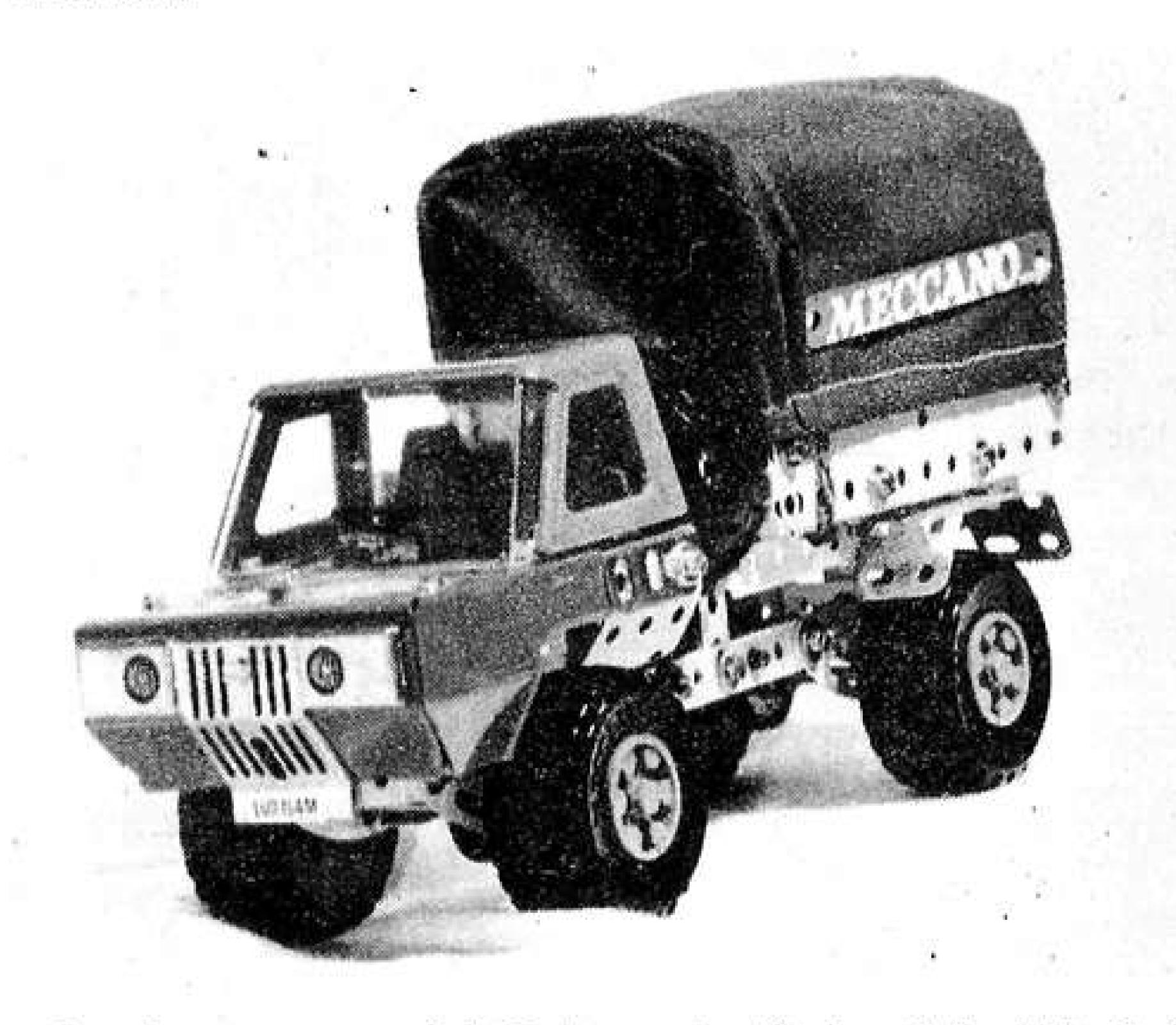
Fig. 2, above: a model Unimog built by Iain Mitchell of Wooburn Green, in which the driving motor is built into the back of the model. In Fig. 3, below, the model can be seen with its 'tarpaulin' cover removed to show the position of the motor and the first stage of the drive, in this case using Bevel Gears.
