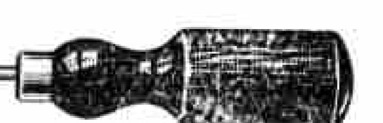
Our illustration shows a type of screw-driver useful for reaching bolts in inaccess-ible places on models. For this reason the blade has been made so that it may be passed through the standard Meccano hole to reach bolts so placed. We are disposing of these screwdrivers whilst our stock lasts, at the special price of 10d. each, post free.
