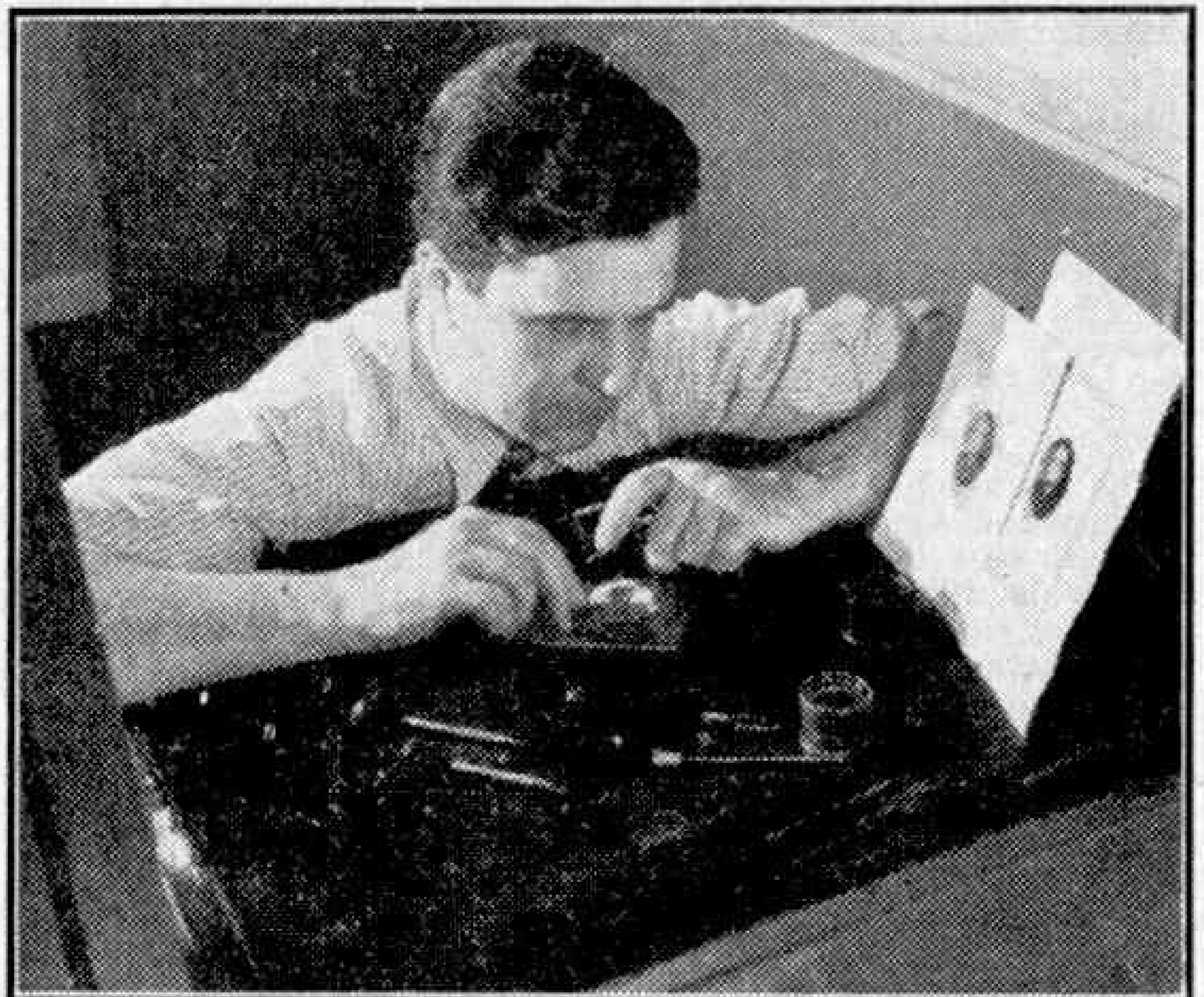
Engraving the steel master die is the first step in the making of a stamp. The engraver cuts the design in soft steel, which is then hardened.
